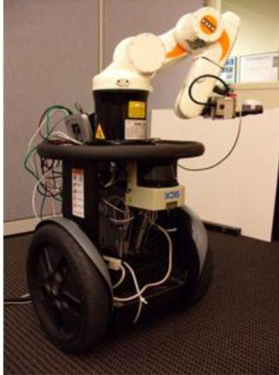
Figure 1. The platform described here, including Segway RMP and KUKA KR5-Sixx.
